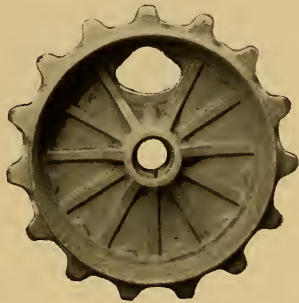
Fig. 25 Tractor Sprocket Wheel— Weight 115 pounds.
